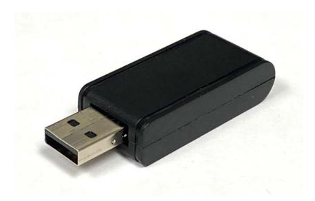
The USB-IR dongle provides a convenient and inexpensive way to correct the clock time and/or reconfigure clock parameters.
